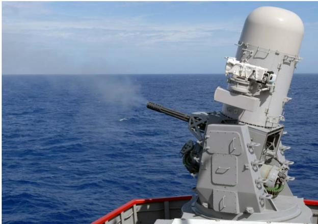
Figure 1. Phalanx Close-in Weapons System (United States Navy Photograph)
